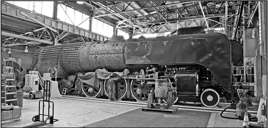
UP 844 “Northern” 4-8-4 is undergoing a complete restoration. Every piece of 844 is being thoroughly inspected and brought back up to the highest standards. The boiler shell has undergone a fresh ultrasound, fresh staybolts and caps have been installed everywhere, and numerous other issues are being corrected. – Photo © 2015 Nathan Zachman.
